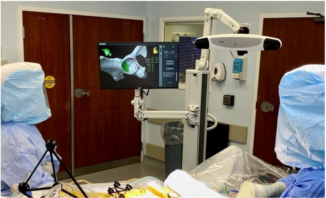
Members of the Doshier Surgical Services Team assist in a Mako robotic hip replacement. The CT planning image on the screen creates a 3D image of the patient's anatomy to create a personalized surgical plan.
